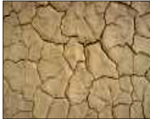
Figure 4-7. Desiccation cracks that form a honeycomb pattern.
