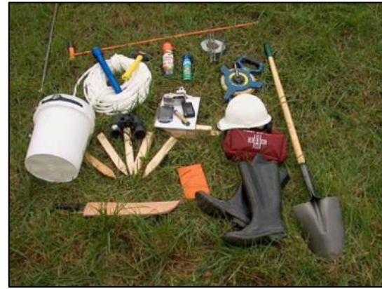
Figure 3-1. Contents of a typical inspection field kit.
