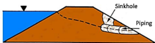
Figure 4-10. A sinkhole caused by a collapse into an animal burrow.
